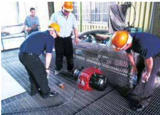
Proof and burst pressure testing
