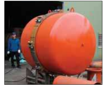
Hydrostatic testing - 72" R-88 coupling
